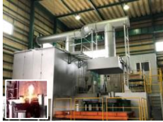
High frequency induction furnace The furnace for experiments or melting on contract. All kinds of analysis are available on the spot.
